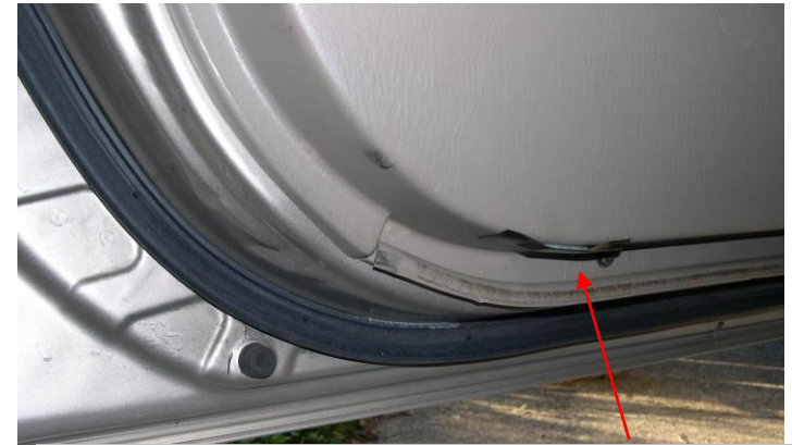
Shows magnet attached in the 2 nd possible place – on the underside of map pocket vs. Inside the map pocket.
